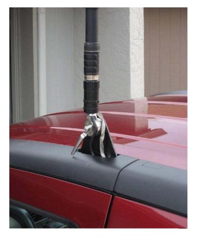
With a 90-degree movement of the handle, the ratchet teeth allow raising of the antenna. It will definitely handle the weight and wind and in about 15 seconds you're mobile. (*Reprinted courtesy eHam.net*) SIGNALS Rockwell-Collins Amateur Radio Club Mail Station 461-290 P.O. Box 833807 Richardson, TX 75083-3807
