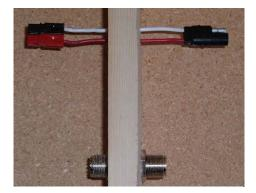
Start by opening the window and measuring the inside width of the window frame. Cut the wood to this length and verify that it's a good fit. Now you can drill the wood for the barrel connector(s). If you need to get other wires outside, you should drill the holes just large enough to pass a single wire through. I suggest drilling them at a downward angle to the outside so that water (from rain or dew) doesn't readily "wick" into the holes.
