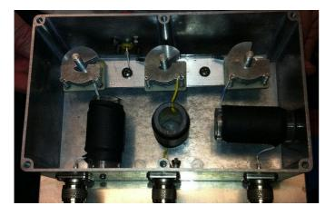
The unit makes use of the band pass filters we've used in past field day exercises and handmade coils and modified variable capacitors. Make sure you thank Dennis and those that have assisted him in the build and test of this special club sponsored Triplexer which may be the secret weapon to this year's ARRL Field Day success. (Submitted by Ross Terry K5SRT)
