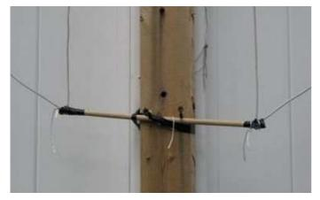
Front to back was around 4 S units. Usable bandwidth is from 7.135 thru 7.185. The ability to work Corsica and then, with a flick of the switch, contact a Columbia, SA station is a lot of fun especially when both stations report a "booming"5-9 plus signal report. Rig is IC 735 with AL 811H at 400 watts.
